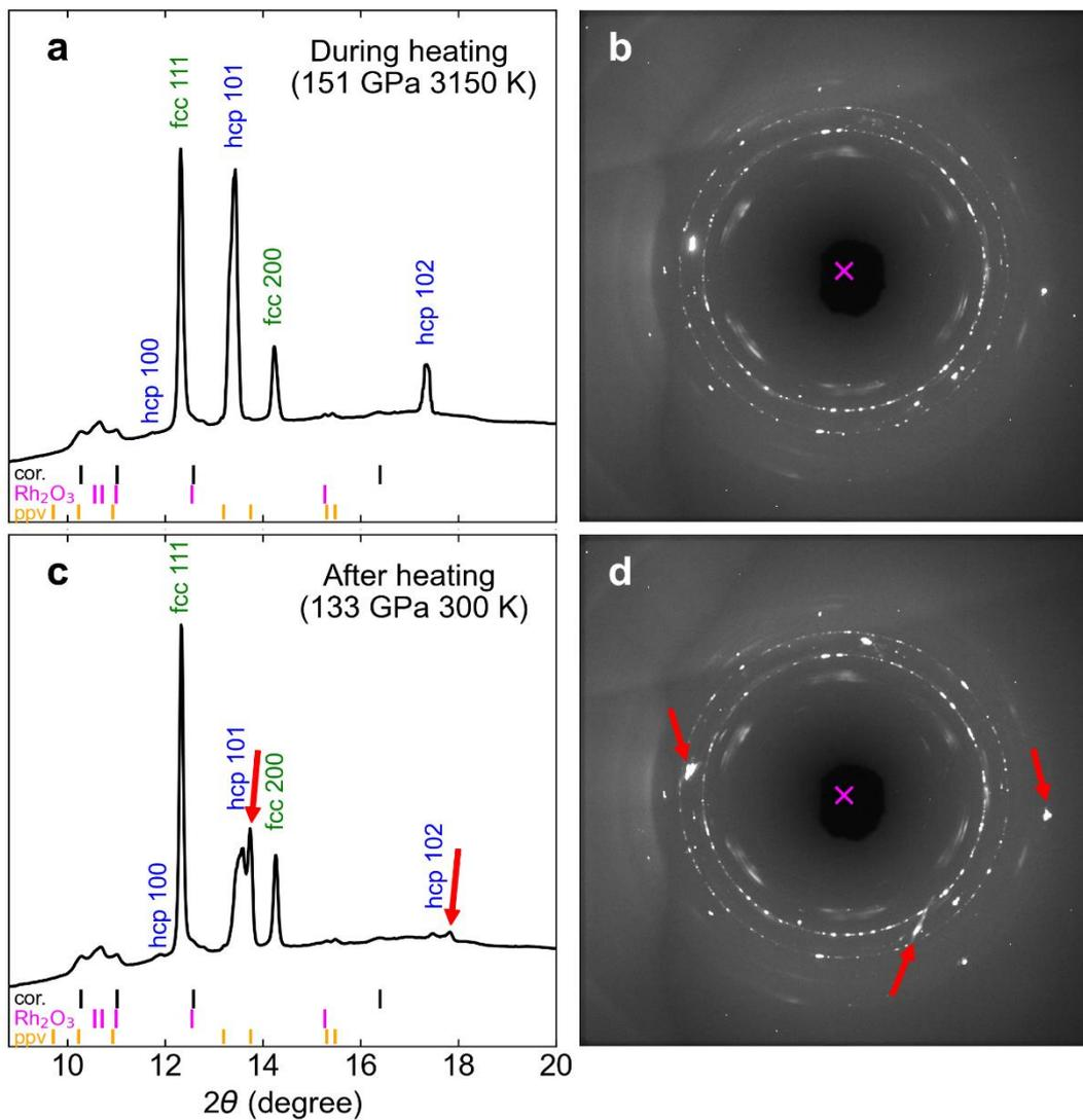
**Figure 4.** 1D and 2D XRD patterns obtained in run #4. Upon gradually decreasing temperature, the diffraction spots from hcp were stretched in the 2D image (marked by red arrows), suggesting the grain growth of the liquidus phase. The peak positions for corundum,  $\text{Rh}_2\text{O}_3$ -type, and post-perovskite-type  $\text{Al}_2\text{O}_3$  are indicated by small bars in (a) and (c).
