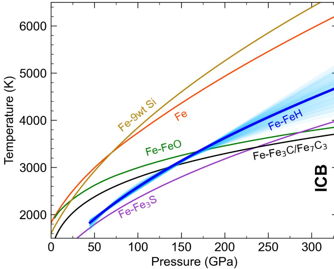
**Figure 7.** Comparison of the Fe-FeH eutectic melting curve with those for other binary Fe alloy systems; Fe-Fe<sub>3</sub>S (Mori et al., 2017), Fe-FeSi (Fe-9wt%Si) (Fischer et al., 2013), Fe-FeO (Oka et al., 2019), and Fe-Fe<sub>3</sub>C/Fe<sub>7</sub>C<sub>3</sub> (Mashino et al., 2019).
