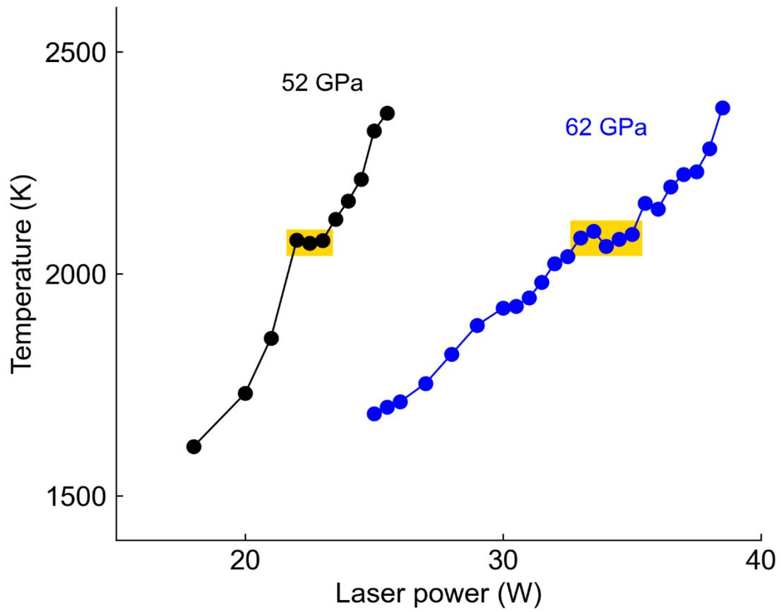
**Figure 1.** Laser power output vs. sample temperature relation. A temperature plateau (yellow part) may indicate melting temperature.
