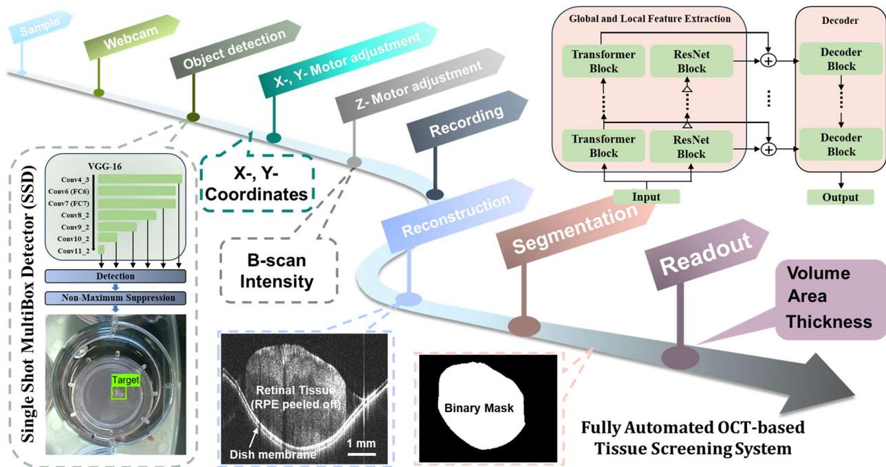
Fig. 2. Pipeline of the fully automated OCT-based tissue screening system.
