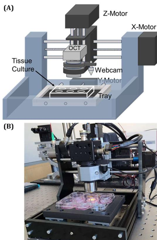
Fig. 1. (a) Schematic diagram and (b) a photograph of custom-designed motorized platform for the automated OCT scan acquisition.
